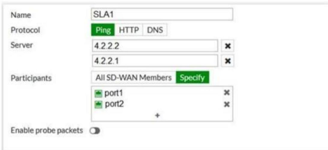
The screenshot shows the configuration for a performance SLA named 'SLA1'. The 'Protocol' is set to 'Ping'. The 'Server' field contains two IP addresses: '4.2.2.2' and '4.2.2.1'. The 'Participants' field is set to 'All SD-WAN Members' with a 'Specify' button. Below this, two ports are listed: 'port1' and 'port2'. At the bottom, the 'Enable probe packets' toggle is turned off.
