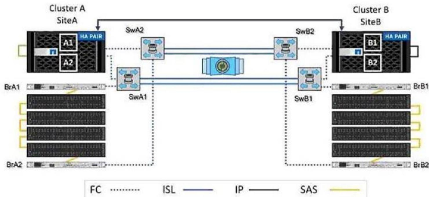
You are investigating an AutoSupport Disk Redundancy Failed alert. Cluster A lost connectivity to storage bridge BrB1, while cluster B lost connectivity to storage bridge BrA1.
