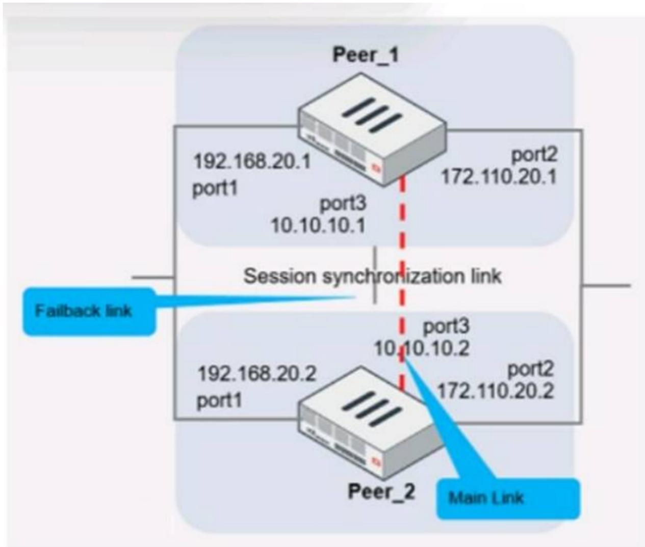
The main link directly connects the two FortiGate devices and is configured using the set session-syn-dev <interface> command.
