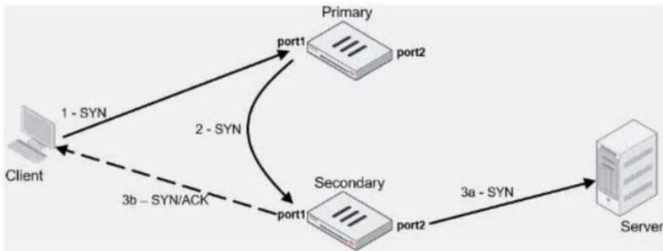
Refer to the exhibit, which contains an active-active load balancing scenario. During the traffic flow the primary FortiGate forwards the SYN packet to the secondary FortiGate. What is the destination MAC address or addresses when packets are forwarded from the primary FortiGate to the secondary FortiGate?
