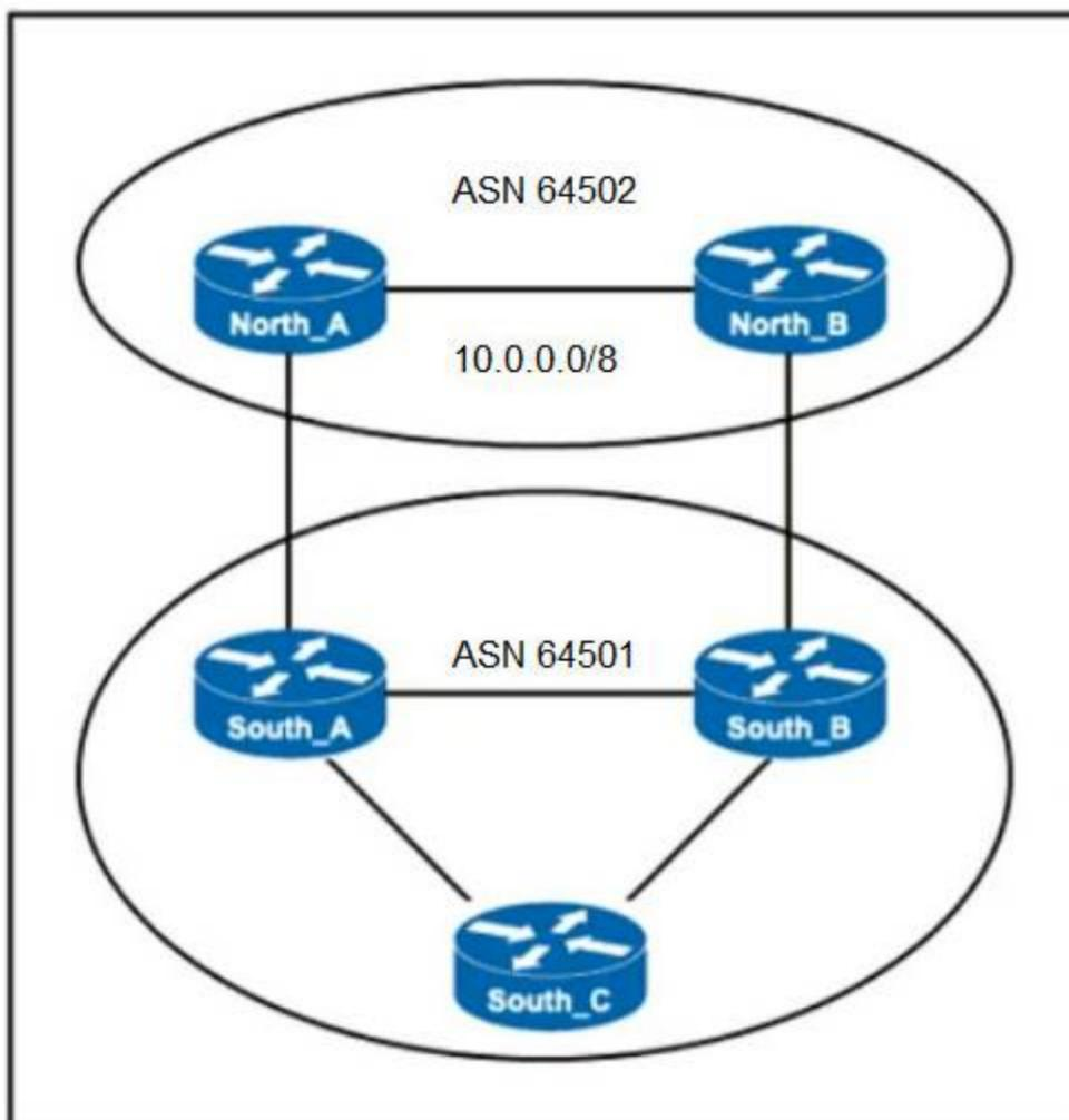
ASN 64501 currently reaches the networks under the 10.0.0.0/8 prefix via the North\_B router, which is a slow backup link. The administrator of ASN 64502 wants traffic from ASN 64501 to 10.0.0.0/8 to travel via the primary link North\_A. Which change to the network configuration accomplishes this task?
