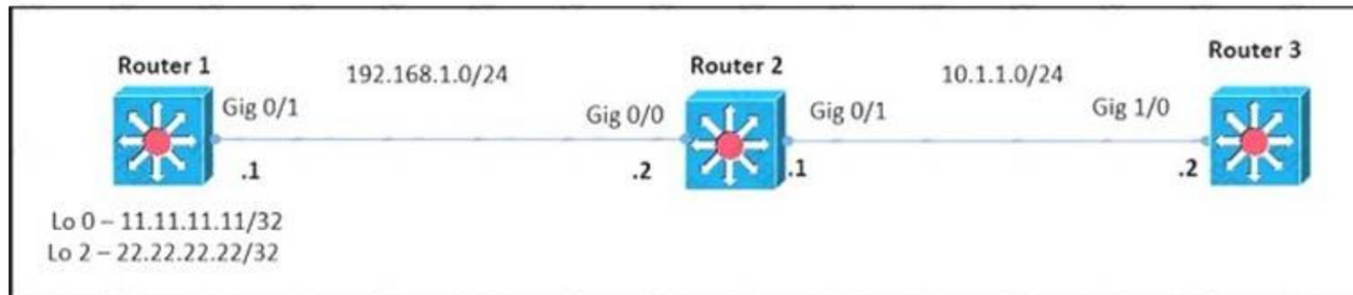
Router 1 and router 2 are running IBGP, and router 2 and router 3 are running OSPF Area 0. Router 1 is advertising loopback interfaces Lo0 and Lo2 and router 2 is redistributing BGP into OSPF Area 0. Which configuration must an administrator apply so that router 2 uses a route map to redistribute only the internal route from Lo 2?
