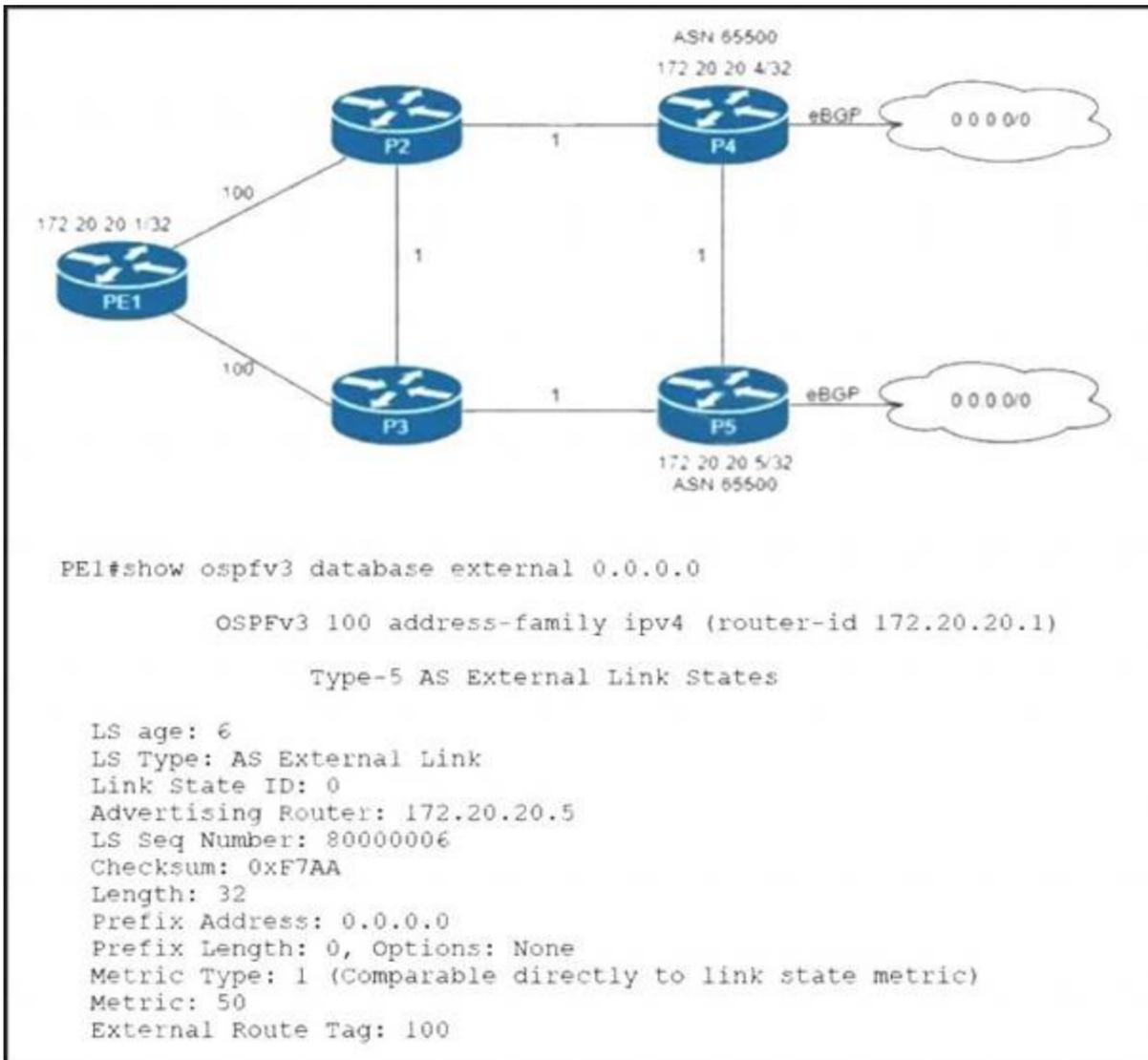
Routers P4 and P5 receive the 0.0.0.0/0 route from the ISP via eBGP peering. P4 is the primary Internet gateway router, and P5 is its backup. P5 is already advertising a default route into the OSPF domain. Which configuration must be applied to P4 so that it advertises a default route into OSPF and becomes the primary Internet gateway for the network?
