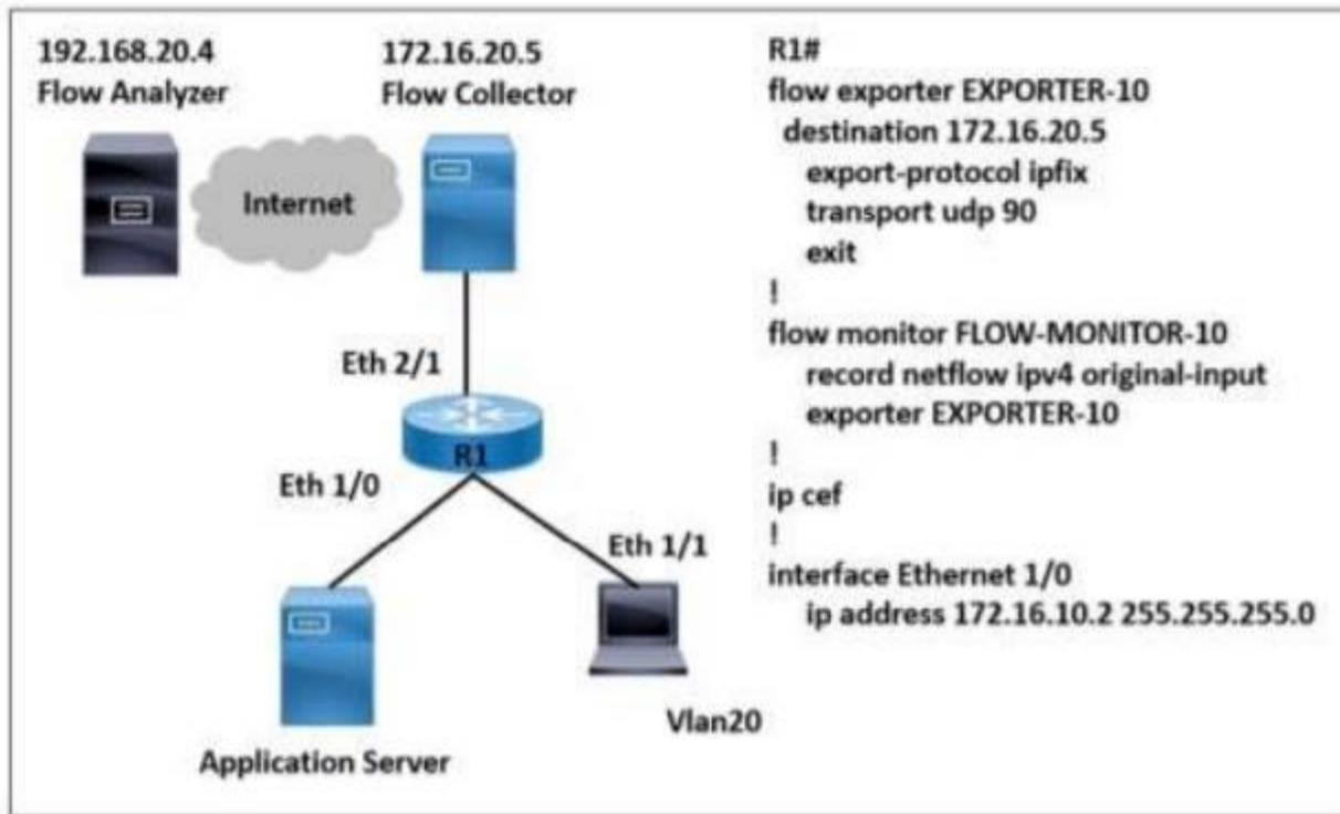
A network engineer wants to monitor traffic from the application server and send the output to the external monitoring device at 172.16.20.5. Application server traffic should pass through the R1 Eth2/1 interface for further analysis after it is monitored. Which configuration must be applied on the R1 router?
