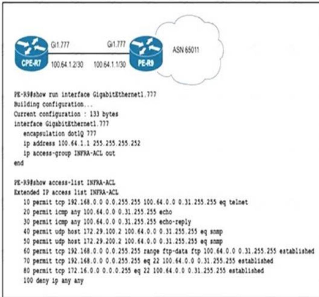
To protect in-band management access to CPE-R7, an engineer wants to allow only SSH management and provisioning traffic from management network 192.168.0.0/16. Which infrastructure ACL change must be applied to router PE-R9 to complete this task?
